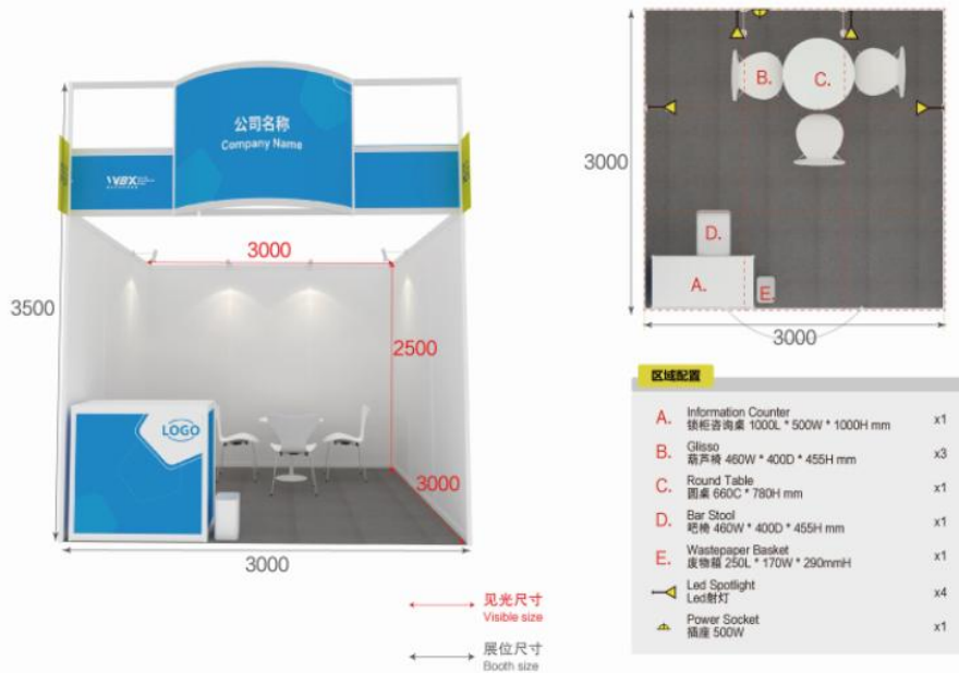
2-01 进阶展台(单开) (3000*3000*3500H) Units: mm INTERMEDIATE SHELL SCHEME
